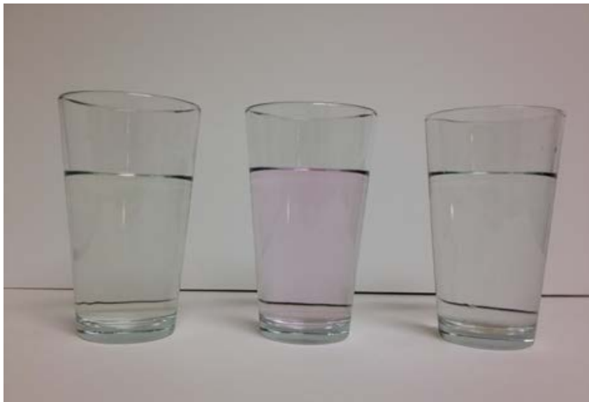
Figure 4-1. Dye concentration comparison (left to right: distilled water, RMZ, and downstream of Riffle 5 at complete mix conditions)
